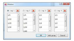
In the dialog box of dilution ratio, after the dilution ration is selected, click ox, the gradient will be displayed in the window. And the related calculation can be performed automatic.
