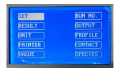
Functions screen includes system setup, testing results, unit setup, printer on and off, values, run no., name output and input, company information and species.
