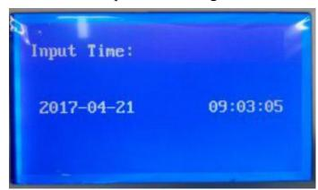
Input time to use number key. If input error, press "Clear" return to main screen and enter again, then input again. After input, press Enter to confirm.
